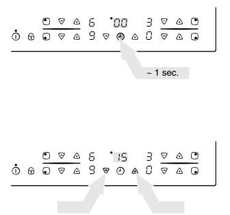
For adjusting the remaining slow cooking time, the required cooking zone must be selected with the Timer sensor field O. The relevant control lamp then flashes quicker. The adjustment is made with the Timer setting senor fields A or  $\bigtriangledown$ .
